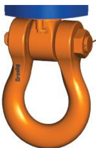
Swivel shackle in selected capacities with bronze thrust or roller thrust bearing
